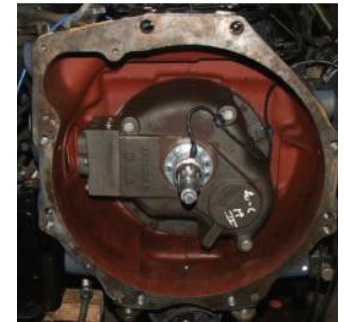
Torductor® sensor fitted to the input shaft on the modified tractor
